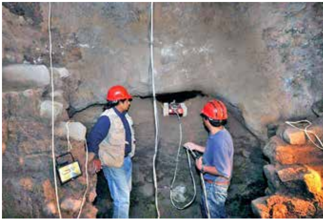
A robot camera is prepared to enter the tunnel located below the Temple of the Feathered Serpent
